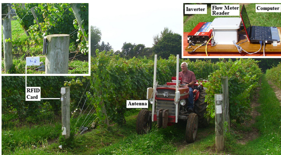
Fig. 14 RFID detection system test in the vineyard
