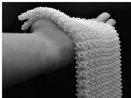
Fig. 12. 3D printed nylon fabric changing its mechanical properties [28]
