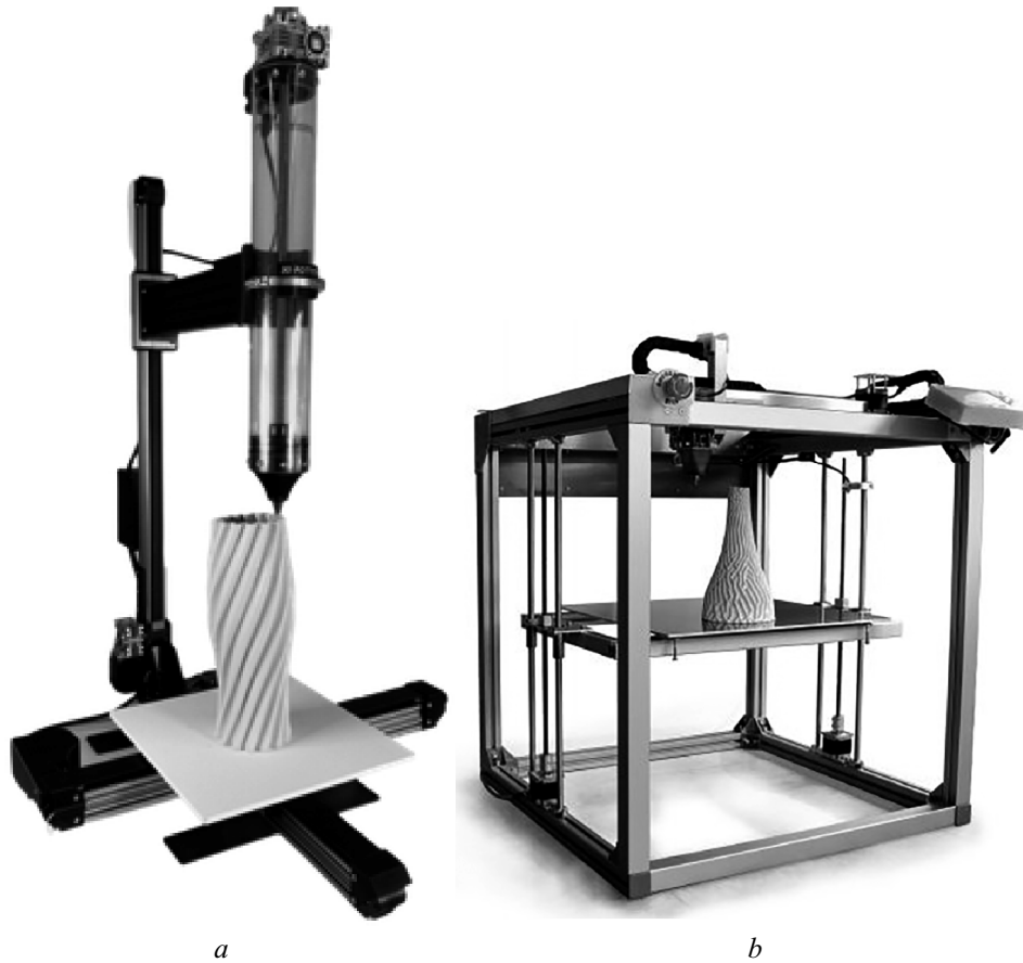
Fig. 10. 3D printers for robocasting: a ) 3D PotterBot 10 XL [21], b ) StoneFlower 3.1 Multimaterial 3D printer [22]
