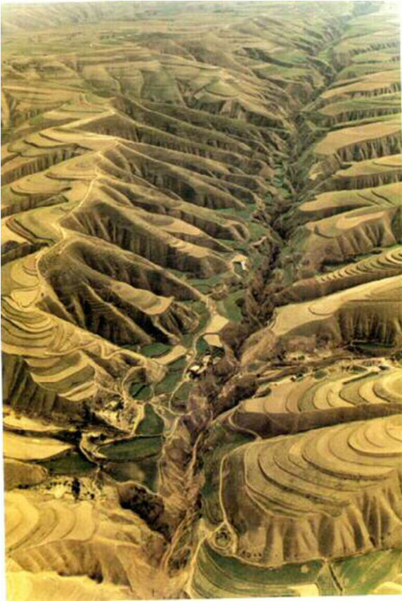
Fig. 2 Aerial photograph of part of the Loess Plateau showing marked erosion and terracing to stabilise the slopes. (Photo courtesy of Dr Xiping Deng, Institute of Soil and Water Conservation, Yangling, Shaanxi, China)
