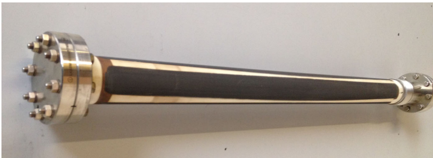
Fig. 1 Thick film electric heating elements deposited on the outside of a vacuum component
