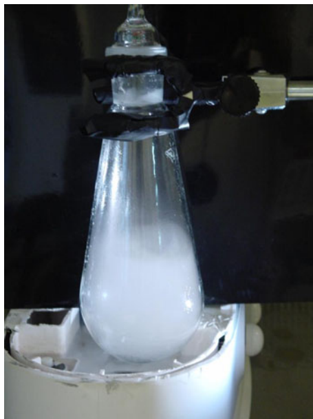
Fig. 2 Aqueous aerosol formed using an ultrasonic generator
