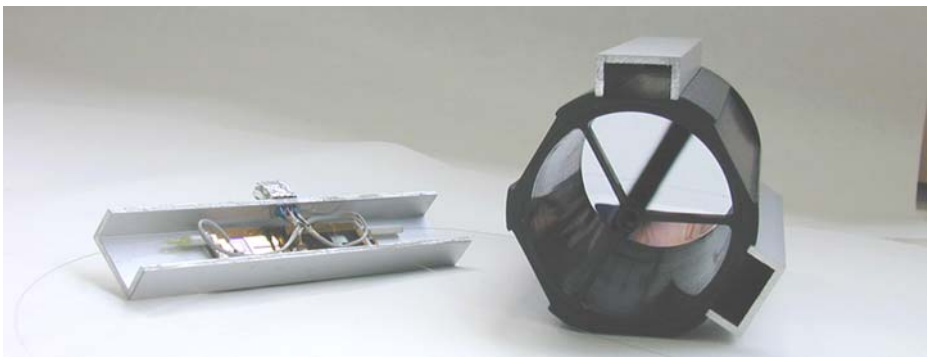
Figure 1 Carbon fibre telescope integrating three interferometers ( right ) together with the detail of a single microinterferometer ( left ).
