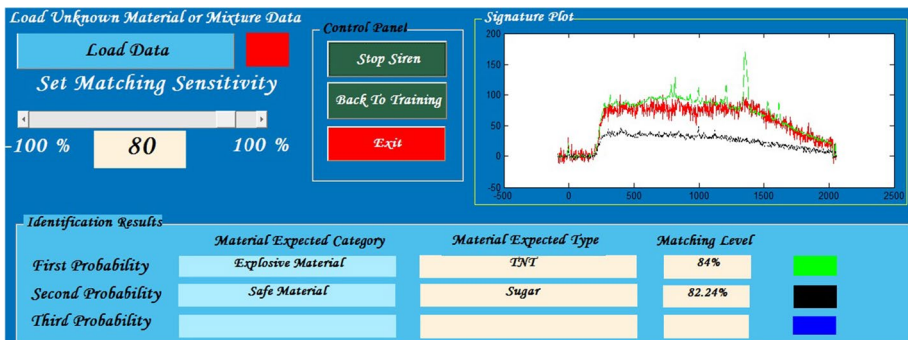
Fig. 26 The recognition interface form shows that the system could identify, classify the mixture of TNT and the sugar with matching levels of 84%, and 82.24%, respectively
