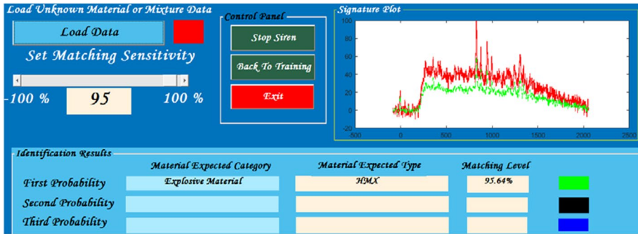
Fig. 19 The recognition interface form shows that the material type is HMX with matching level of 95.64%
