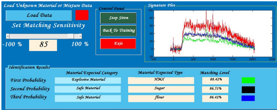
Fig. 24 The recognition interface form shows the identified substances, the classification, the signature plot (on the top right part of the figure), and the matching levels of the substances form the mixture
