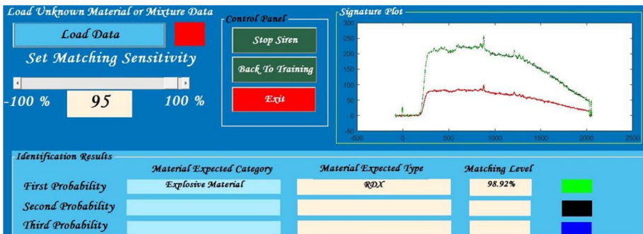
Fig. 22 The recognition interface form shows that the material type is RDX with matching level of 98.92%
