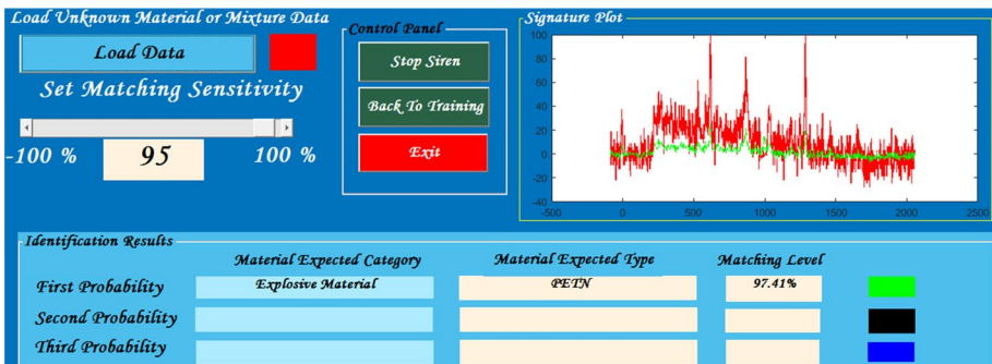
Fig. 18 The recognition interface form shows that the material type is PETN with matching level of 97.41%
