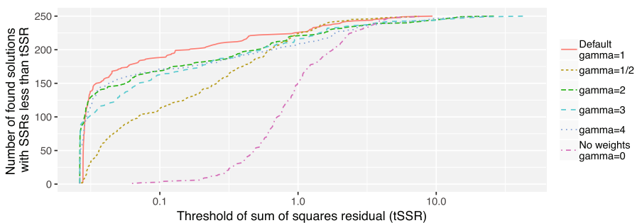
Fig. 10 Number of minimisers found for given accuracy threshold (tSSR) using various weights for the linear approximation (i.e., various \gamma ). Smaller SSR indicates more accurate solution to the nonlinear-least squares problem
