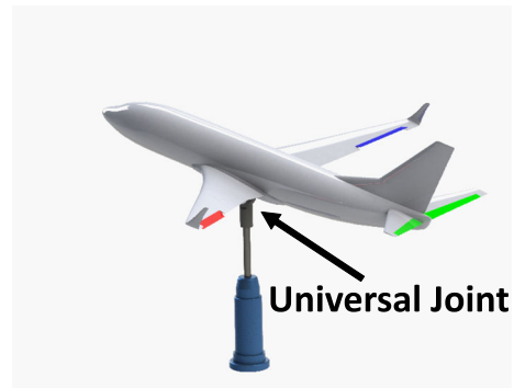
Fig. 4 A schematic for a two-DOF pitch-roll wind tunnel model for testing the LIBRA mechanism
