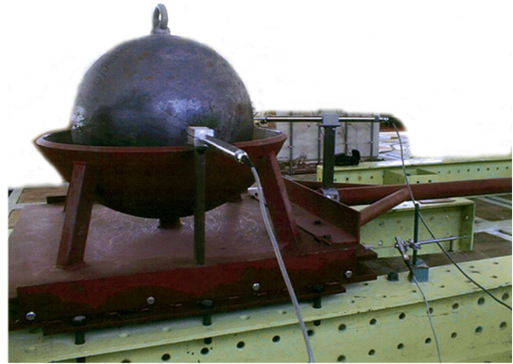
Fig. 1 Ball vibration absorber in a dynamic testing laboratory
