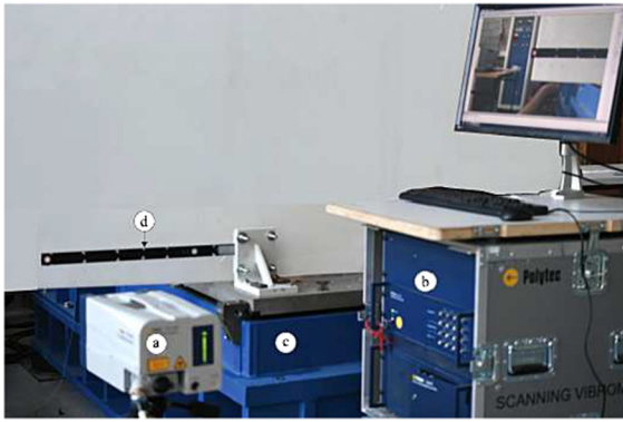
Fig. 3 Experiment setup; a laser scanning head with camera, b computer with scanning unit, c anti-vibrational table, d composite specimen
