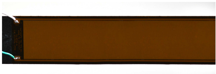
Fig. 4 Section of the MFC patch (orange colour) bonded onto the composite specimen (black). (Color figure online)
