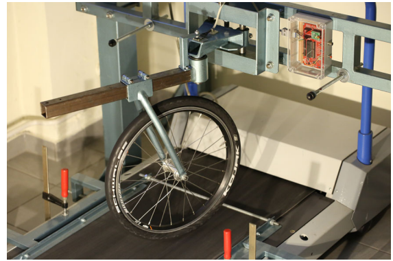
Fig. 10 Shimmying wheel running on a conveyor belt. (Colour figure online)
