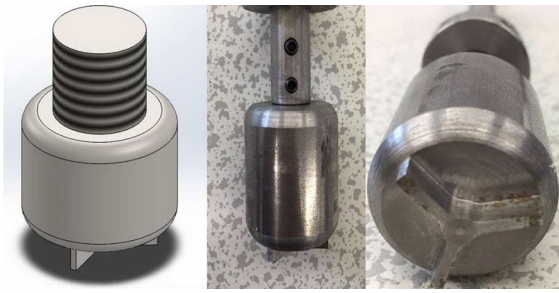
Fig. 6 Drill-bit Solidworks drawing (left), photograph of the drill-bit (middle), and photograph of the drill-bit's tri-blade design (right)
