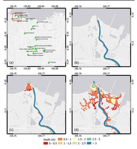
**Fig. 12** Depth and extent of flooding around the West Flood Canal and Muara Angke river inlet from Q100 river discharge combined with coastal storms. **a** A map of Jakarta showing the modelled area in red; **b** no coastal storm and 0 m surge (baseline scenario); **c** W1 and 0 m surge; **d** W100 and 0 m surge
