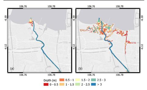
Fig. 13 Depth and extent of flooding around the West Flood Canal and Muara Angke river inlet from Q100 river discharge combined with coastal storms a W1, b W100, and 1 m surge
