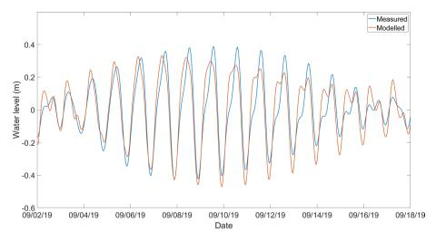
Fig. 5 Validation of Jakarta Bay hydrodynamic model against measured water level data by Ancol tide gauge located at Jakarta Bay during the period from 01/09/2019 to 18/09/2019
