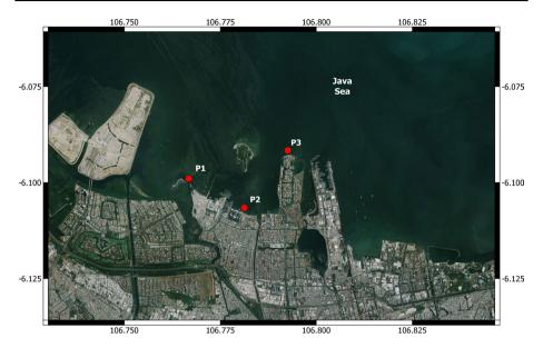
Fig. 9 Individual output point locations selected to closely examine wave heights and water levels along the south-east shoreline of Jakarta Bay
