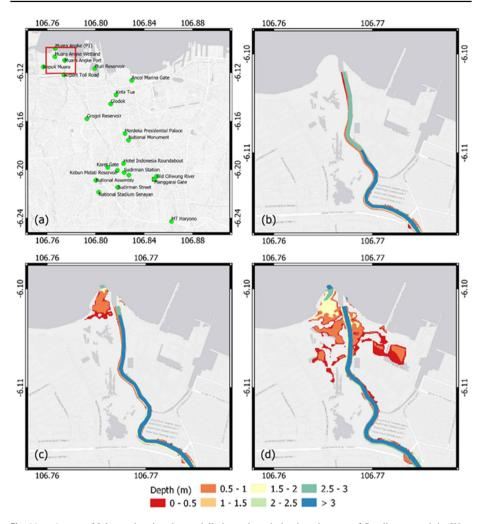
**Fig. 11 a** A map of Jakarta showing the modelled area in red; depth and extent of flooding around the West Flood Canal and Muara Angke river inlet from Q2 with **b** no coastal storm and 0 m surge (baseline scenario); **c** W1 and 0 m surge; **d** W100 and 0 m surge
