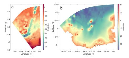
Fig. 4 Delft3D numerical model domains and model bathymetry of Jakarta Bay. a Large scale domain; b high-resolution small, nested domain of Jakarta Bay
