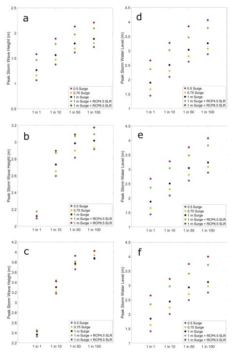
Fig. 10 Peak storm wave heights (a-c) and peak storm water levels (d-f) at P1, P2 and P3, respectively
