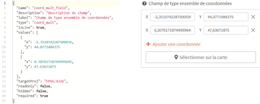
Fig. 5 Relation between the JSON configuration file stored on the gitlab and the corresponding boxes on the User Web Portal
