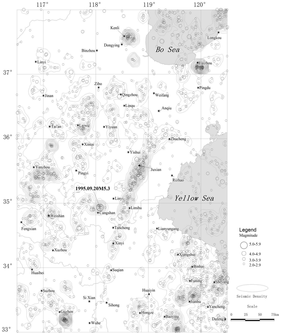
Fig. 3 Plot of the epicenters of events of different magnitude and contours of the seismic density index defined in Eq. 1 ( M_{Lmin} = 2.0 ). The values of contours start from I_{j,t} = 1 and increase in unit steps
