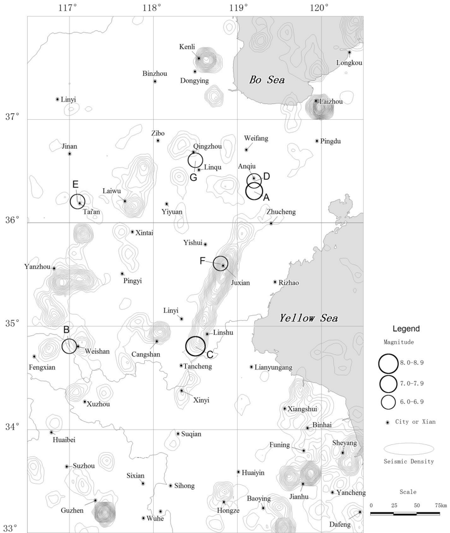
Fig. 4 Plot of the epicenters of strong historical earthquakes with M_s \geq 6 , and contours of the seismic density ( M_{Lmin} = 2.0 ). The source parameters of the strong historical earthquakes shown in circles are listed in Table 1. The values of contours start from I_{j,t} = 2 and increase in unit steps
