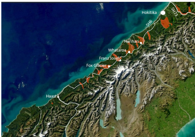
Fig. 11 Floodplains in Westland (orange) potentially vulnerable to post-seismic aggradation following the next major earthquake in the region. White line = State Highway 6
