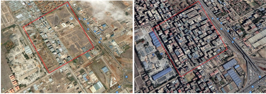
Fig. 11 The evolution of residential buildings in Embakasi pipeline estate (point d) in Fig. 7. The image on the left illustrates the distribution of residential units before 2010 while the image on the right illustrates the current distribution. The red outline illustrates the extends of the current land subsidence. The images were taken from Google Earth
