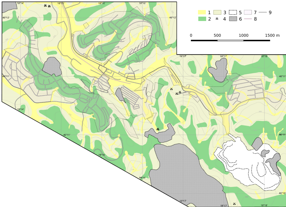
Fig. 4 The geomorphologic map of the town of Komló (CSK); 1 = valley, 2 = ridges 3 = slopes, 4 = closed coal mine, 5 = andesite quarry, 6 = mine dumps, 7 = residential areas, 8 = railway, 9 = road
