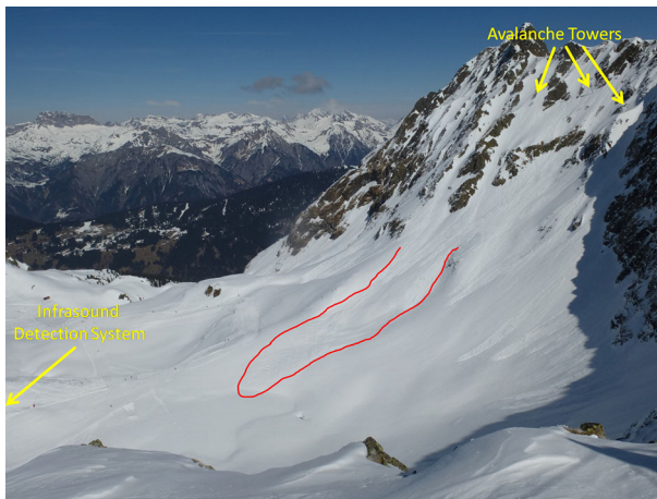
Fig. 14 Picture of the deposit zone ( red line ) of the avalanche at 03.03.2015 and position of avalanche towers (the left three of five) and the single sensor detection system
