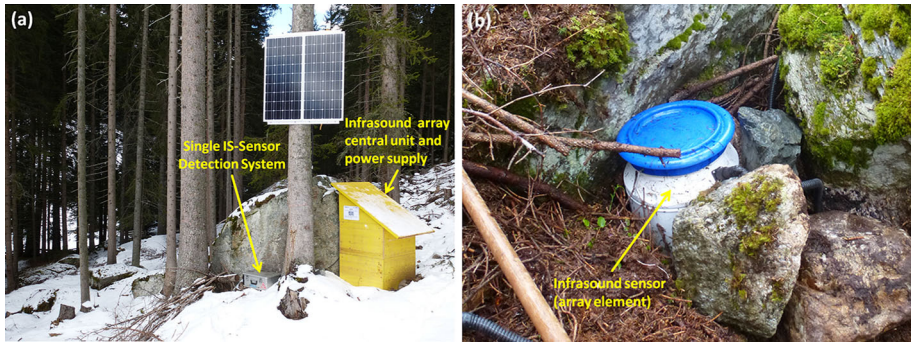
Fig. 4 Set-up of the infrasound array at Ischgl. a Central unit of the array with power supply and place of single sensor system in the first year (2013/2014). b One of the four infrasound sensors of the array
