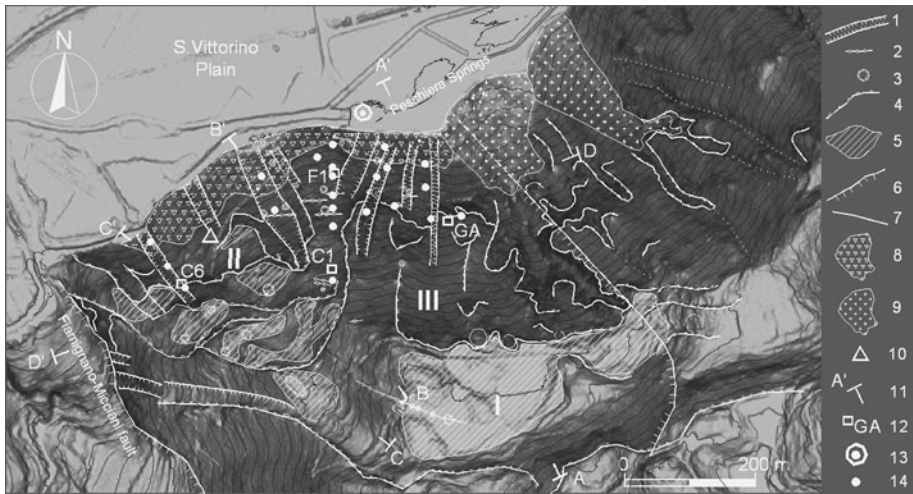
Fig. 4 Digital elevation model (DEM) based on the LIDAR remote survey showing geomorphological features; the traces of the geological sections of Fig. 3 are also shown. (1) Trench; (2) Tension crack; (3) Sinkhole; (4) Scarp; (5) Karstified flat; (6) Fault; (7) Gully; (8) Slope debris; (9) Debris fan deposit; (10) Location of the rock fall of 22 March 2011 recorded by the accelerometric network at the plant; (11) Trace of the geological cross-sections (see Fig. 3); (12) Accelerometric station at the drainage plant; (13) Reference point for the azimuthal distribution of the time integral of the square velocity, derived from seismic noise records; (14) Velocimetric station for measuring seismic noise at the drainage plant. Slope sectors (I, II and III) at different evolutionary stages are also shown
