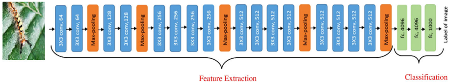
Fig. 2 A visualization of the VGG architecture
