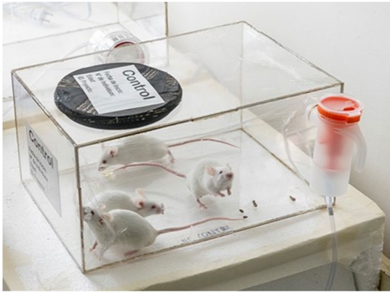
Fig. 2 Biomodels exposed to negative control (0.9% saline solution), using a whole-body inhalation chamber
