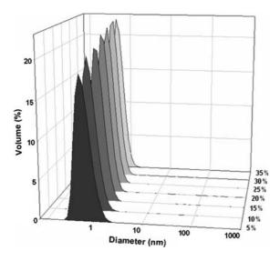
Fig. 4 Volume particle size distributions obtained for different sucrose concentrations measured on a Nano S instrument using backscatter detection
