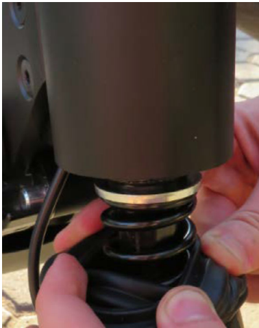
(a) Front suspension of the SEAT eXS Kick scooter ES2
