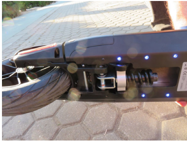
(a) Rear suspension of the SEAT eXS Kick scooter ES2
