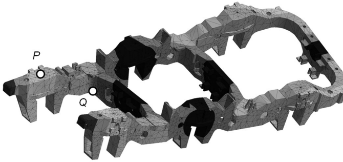
Fig. 11 Overview of the first flexible mode of vibration of the bogie frame
