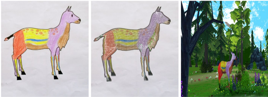
Fig. 10 Drawing used as 3D texture: the drawing, the mapping, and the animal with the texture in the 3D environment
