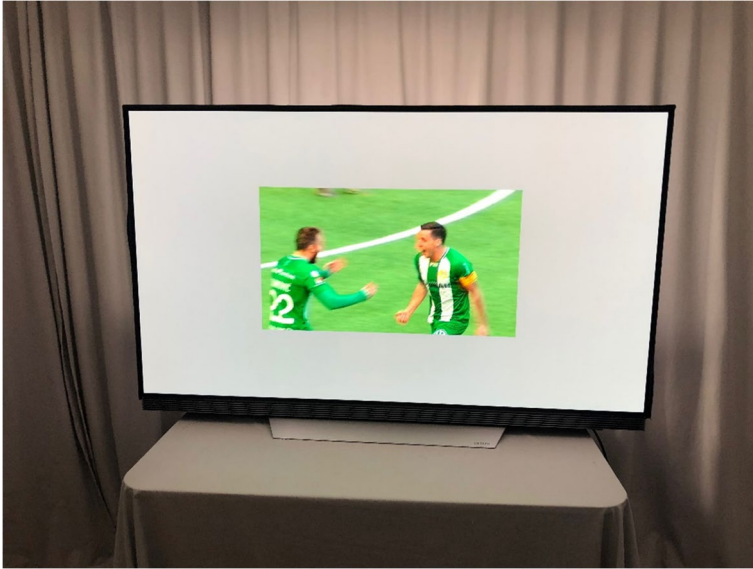
Fig. 4 The video with resolution 1920 \times 1080 pixels was presented in the centre of the screen with a grey surround
