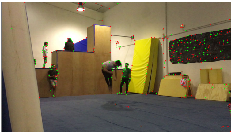
Fig. 4 Example of well-known BG key points filtering. Red represents well-known BG key points while green represents the remaining set of key points
