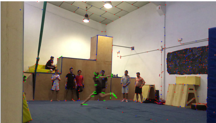
Fig. 5 Example of motions estimated using a pyramidal implementation of the Lucas-Kanade algorithm. In green the set of motion vectors associated to FG key points, in blue those with very small magnitudes, and in red well-known BG key points
