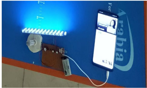
Fig. 12 Practical transmitter circuit
