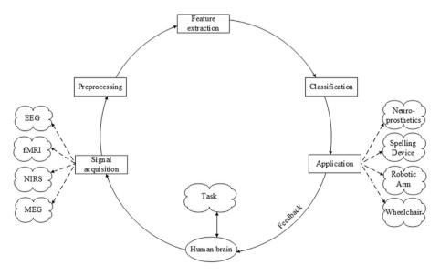
Fig.4 Typical BCI components
