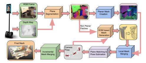
Fig. 2 The block diagram of our proposed pipeline of robust 3D scene reconstruction from the robot's ego view (RGBD sensor)
