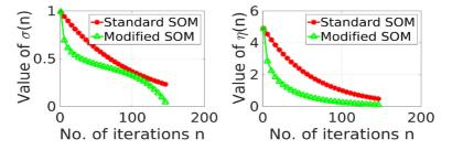
**Fig. 6** Comparing the modified vs. the convention decay functions for  $\sigma$  (left) and  $\eta$  (right). Notice that during the initial and towards the end of iterations the modified  $\sigma$  decreases faster. The value of modified  $\eta$  is also less in the ordering phase compared to the conventional one
