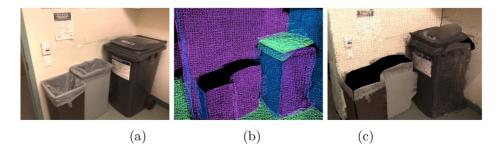
**Fig. 1** 3D Mesh generated by proposed pipeline on Copyroom [16] dataset. (a): original frame, (b): generated normal wire-frame, (c): vertex-colored 3D mesh
