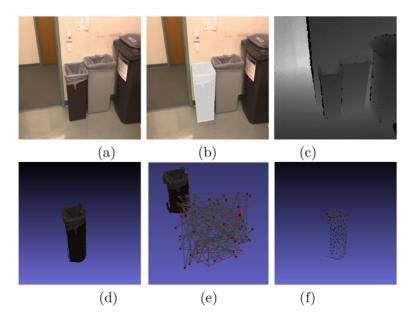
**Fig. 4** Different steps of non-planar mesh approximation given an RGBD image. (a): Input RGB image of the scene, (b): object segmentation, (c): depth map, (d): point-cloud of the object extracted from the scene RGB of (a), segmentation mask of (b) and depth map of (c), (e): initialization of the mesh nodes and (f): approximated mesh
