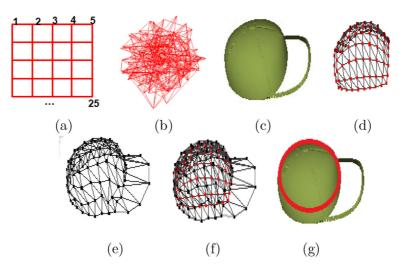
**Fig. 5** Showing boundary effect due to conventional SOM and the proposed SOM. (a): Schematic diagram depicting a 2D 5  $\times$  5 lattice of mesh nodes (the numbers represent the node index), (b): condition of 10  $\times$  10 mesh after initialization, (c): input cap point-cloud, (d): result of applying conventional SOM, (e): result of applying proposed Algorithm 2, (f): (e) overlayed on (d), (g): (d) and (e) overlayed on (c), the red curve shows the boundary of (d)
