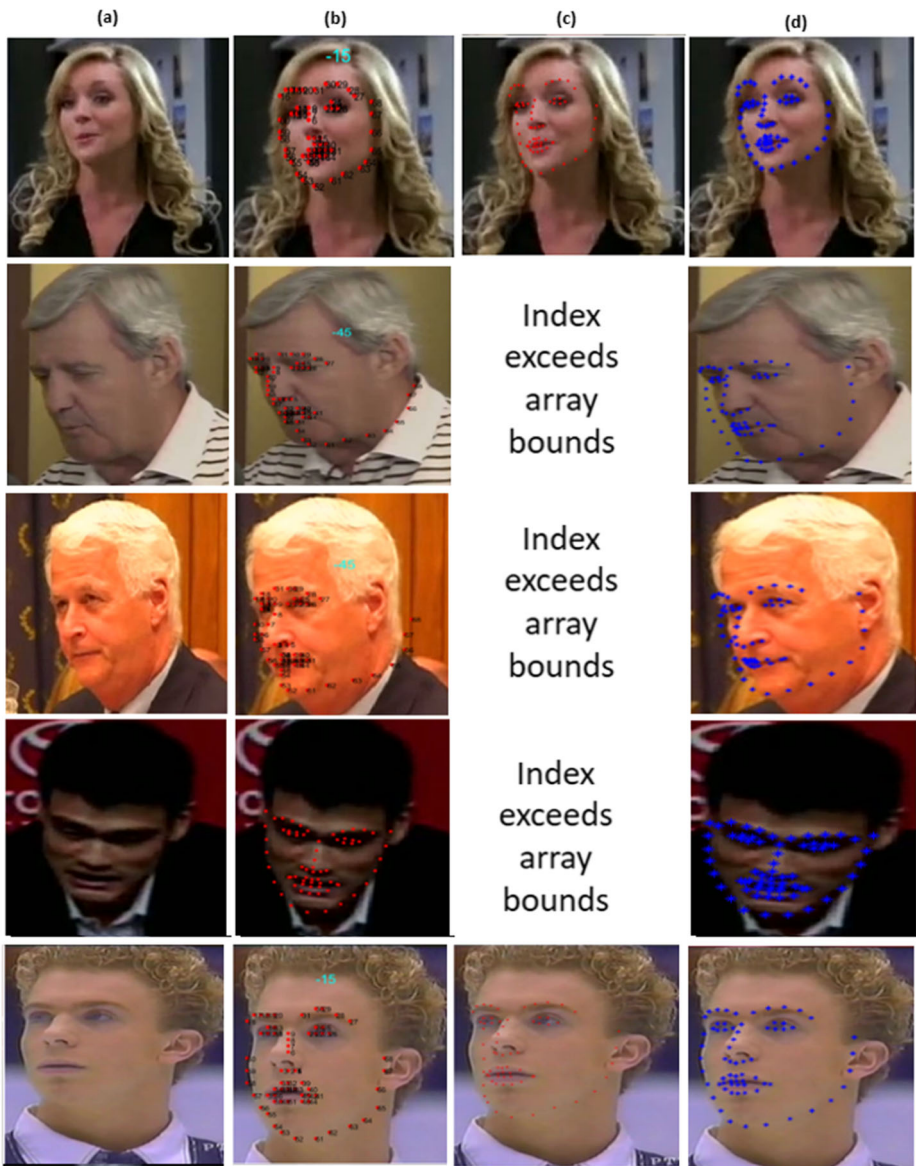
Fig. 16 68 facial landmarks detection: (a) Input face image, (b) 68 landmarks detection using Chow-Liu algorithm, (c) 68 landmarks detection using the Gaussian-Newton method, (d) 68 landmarks detection using dlib and OpenCV
