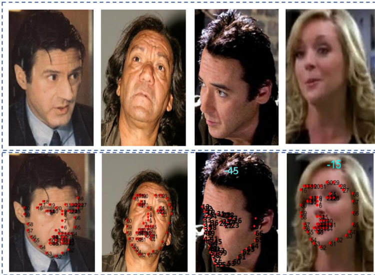
Fig. 8 68 landmarks detection using dlib library: First row: input face images, Second row: numbered 68 landmarks
