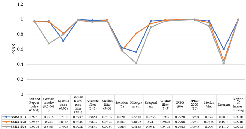
Attacks Fig. 11 Comparison of SSIM values for P1, P2, and P3 (various attacks)
