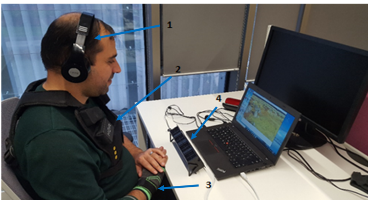
Fig. 1 Experimental setup. The users were wearing: (1) i-Shine headphone ( https://www.ishine-trade.com ), (2) the KOR-FX haptic vest ( http://www.korfx.com/ ) (3) Mio Link ( https://www.mioglobal.com/ ) (4) olfactory effects were diffused using Exhalia ( https://www.exhalia.com/ )
