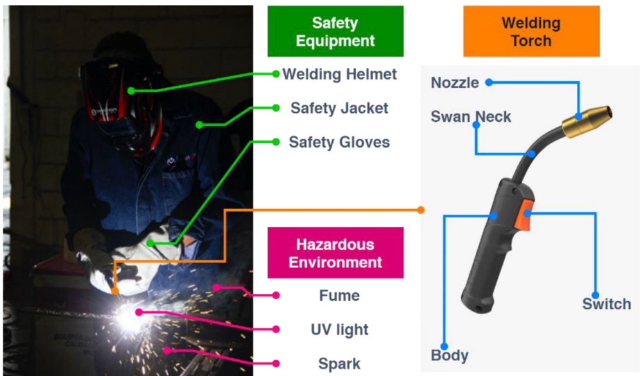
Fig. 1 The welder is wearing safety equipment and holding a welding torch to do the welding task
