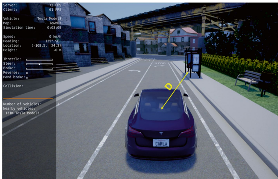
Fig. 12 Unexpected Pedestrian scenario. The pedestrian can be found behind the bus stop, so the perception systems detects it at the moment it is entering the road
