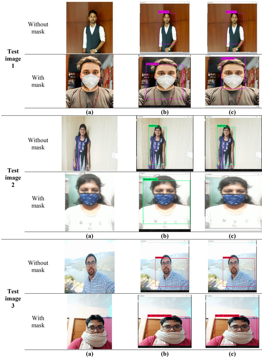
Fig. 15 Experimental results on some sample images a Original image b Detection results by YOLOv3 c Detection results by YOLOv3-tiny
