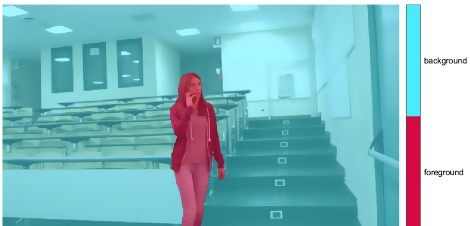
Fig. 2 A label overlay of a training image. The background pixels (light blue), are more frequent with respect to the foreground pixels (red). The frequency of foreground pixels in the training dataset is 11.16%, and the frequency of background pixels is 88.84%
