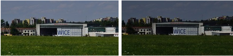
Fig. 14 On the left: shutter speed calculated by ESAM algorithm with \alpha = 0.5 , percentage of black/white pixels: 0.0/0.0; on the right: shutter speed calculated by ESAM algorithm with \alpha = 0.1 , percentage of black/white pixels: 3.1/0.0
