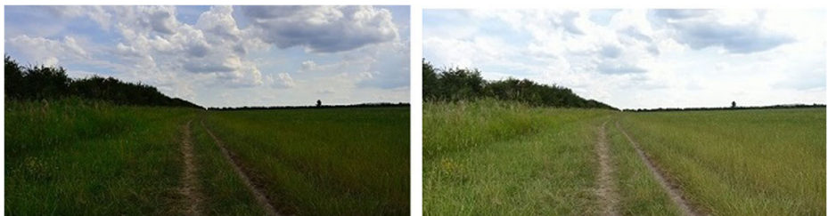
Fig. 13 On the left: shutter speed calculated by ESAM algorithm, percentage of black/white pixels: 0.0/6.8; on the right: image taken by Nikon D3100's automatic exposure mode, percentage of black/white pixels: 0.0/29.8
