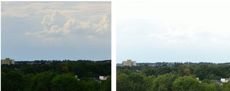
Fig. 12 On the left: shutter speed calculated by ESMV algorithm, percentage of black/white pixels: 10.1/0.0; on the right: image taken by Nikon D3100's automatic exposure mode, percentage of black/white pixels: 0.0/17.6
