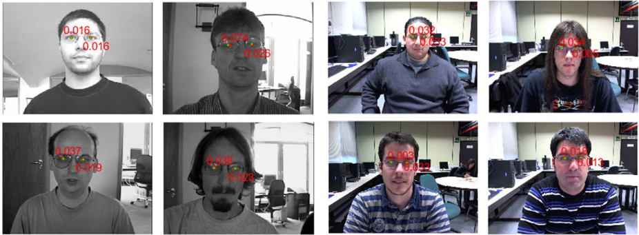
Fig. 7 The qualitative results on the objects with glasses of the BioID and GI4E database. (The red points represent the estimated eye center positions by our proposed approach. And the green points represent the ground truth. The normalized error of each eye center is also labeled in red.)
