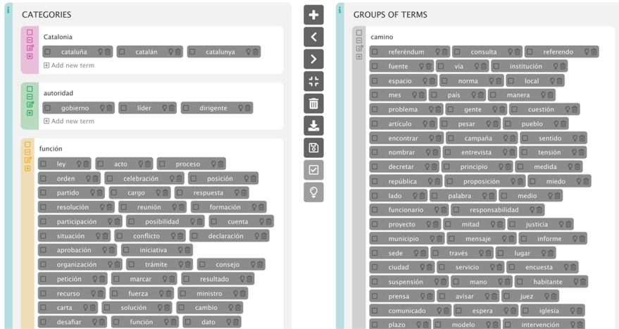
Fig. 6 Term categorization (step 3): the users can explore the groups of terms generated automatically (right panel), modify them (central panel), and include them to the final version of the taxonomy (left panel)
