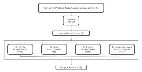
Fig. 1 Architecture of the AVISPA tool
