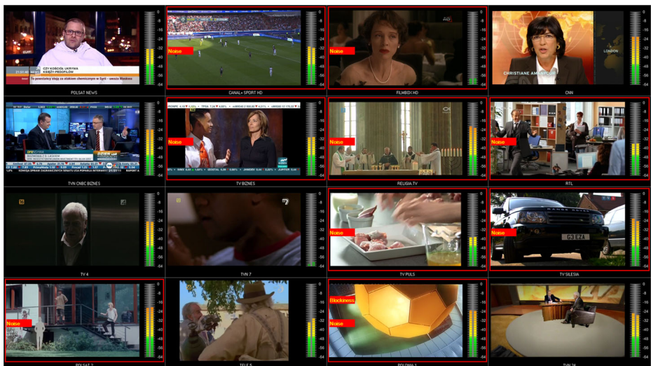
Fig. 8 Example of screens of NET-MOZAIC showing the alarms. Alarms are displayed as color (yellow or red) frames around the channel window. The name of the metric causing the alarm appears as text on the red or yellow bar
