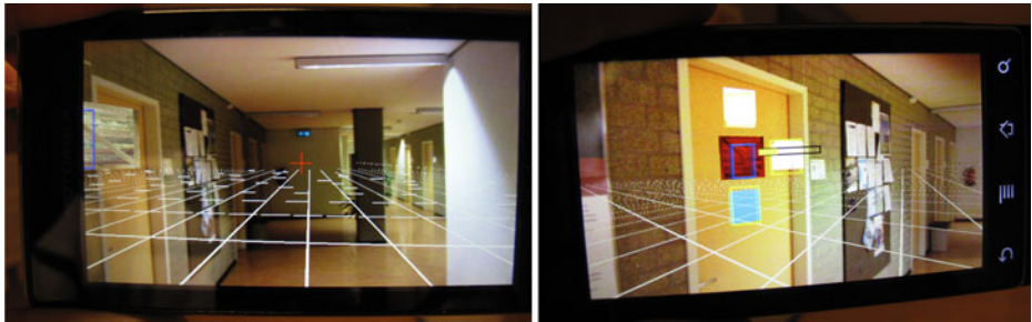
Fig. 6 Device based interaction: selection by pointing a reticule ( left ) to the target till the related bar is filled ( right )
