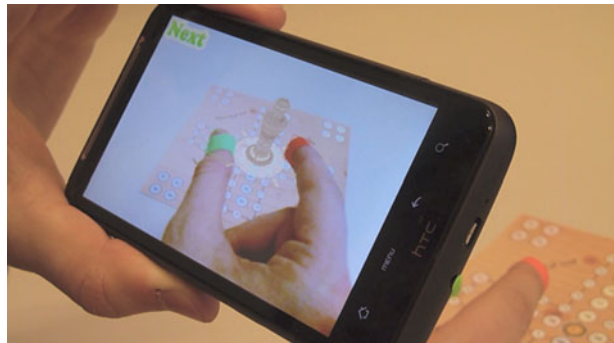
Fig. 14 A green marker ( thumb ) and a red one ( index finger ) are used to track fingers and manipulate virtual objects on the board game
