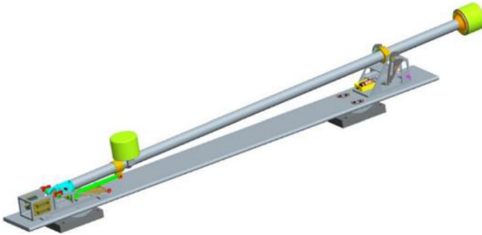
Fig. 8 Example of developed and tested boom with two flux-gate magnetometers for the KOMPSAT mission
