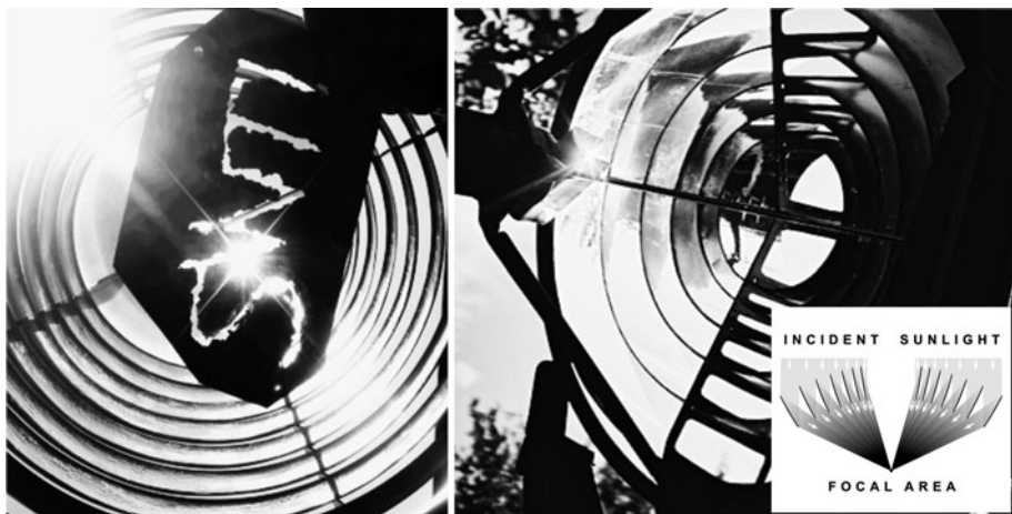
Fig. 3 Prototypes of ring-array solar concentrating collectors under field testing. An example of ray-trace diagram illustrating the operating principle of optical scheme of the RAC is shown in the lower-right corner
