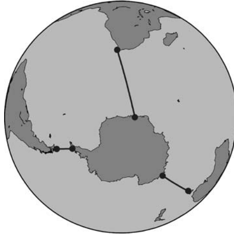
Figure 6. Examples for links between tide gauges (crossing the Antarctic Circumpolar Current), for which high precision geoid differences are required for ocean circulation modelling.
