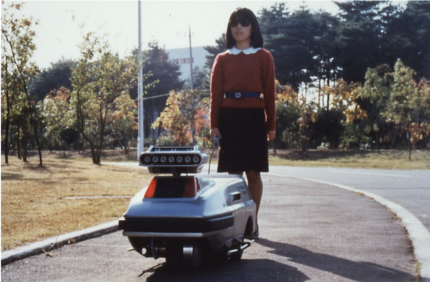
Fig. 1 Guide Dog Robot, MELDOG Project from the TachiLab (see Guide Dog Robot (MELDOG) from TachiLab, https://tachilab.org/projects/meldog.html )
