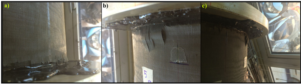
Fig. 8 Highlights from compression tests on CFRP skirts showing the specific damaging mechanisms due to compression load
